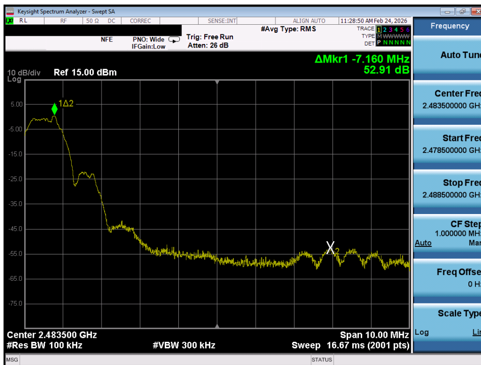
Plot 7-25. Band Edge Plot (ANT+ – Ch. 78)
