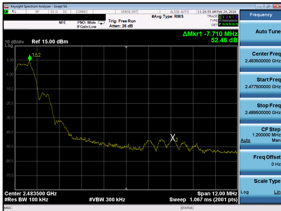
Plot 7-24. Band Edge Plot (ANT+ – Ch. 77)
