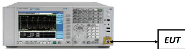
Figure 7-4. Test Instrument & Measurement Setup
