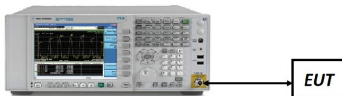
Figure 7-3. Test Instrument & Measurement Setup
