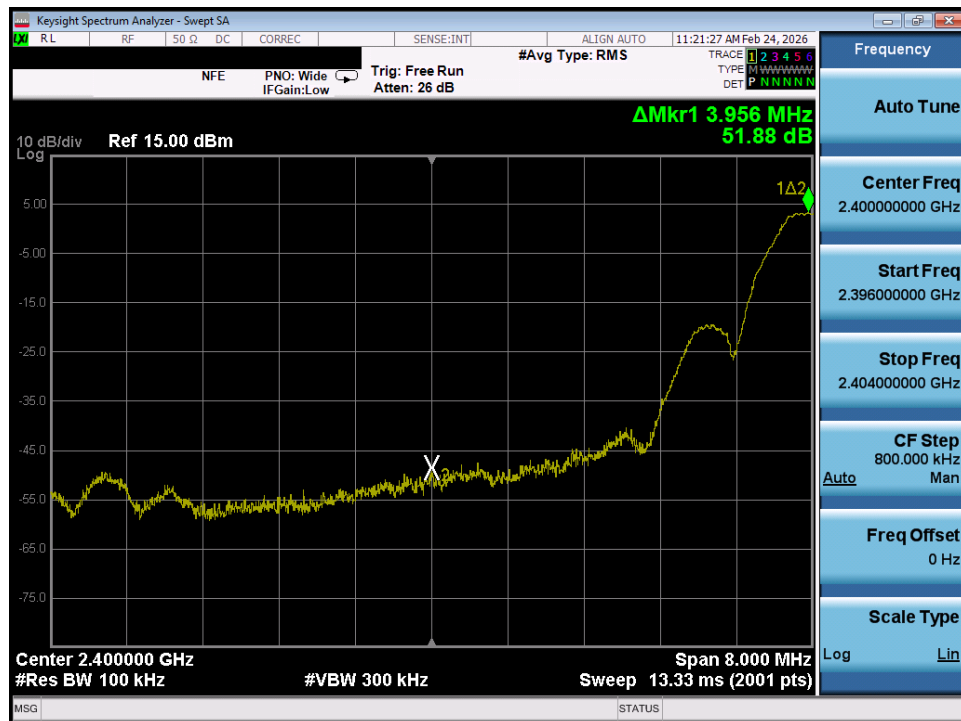
Plot 7-23. Band Edge Plot (ANT+ – Ch. 3)
