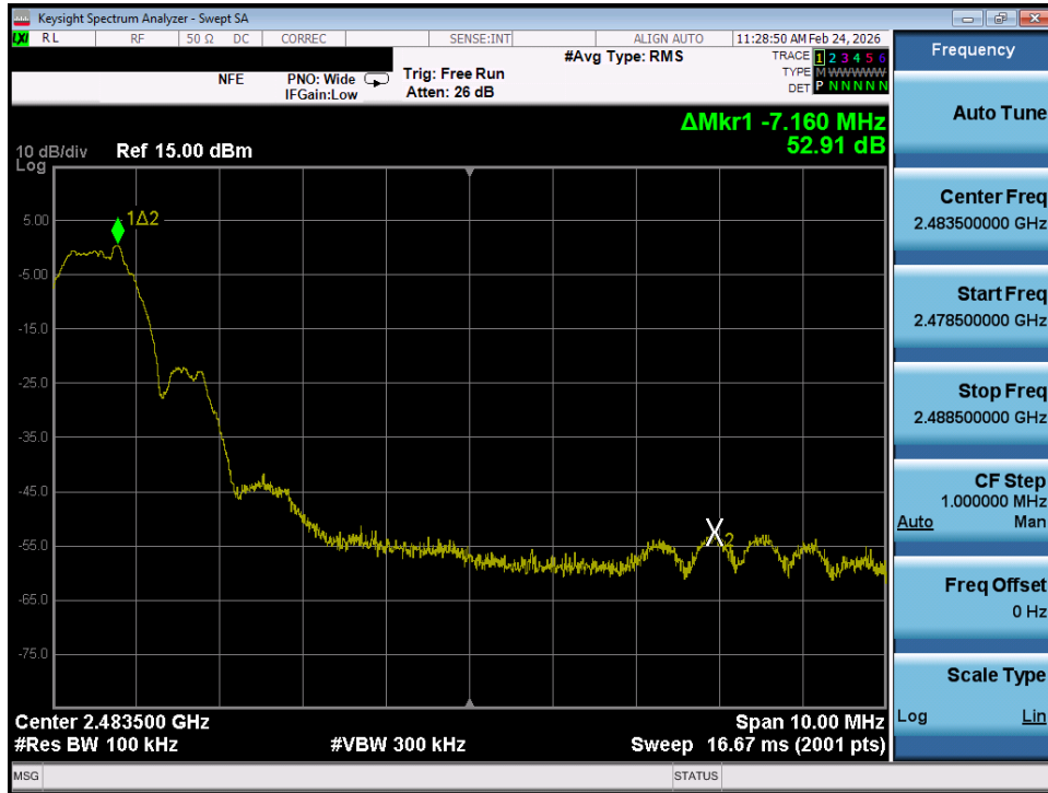
Plot 7-25. Band Edge Plot (ANT+ – Ch. 78)
