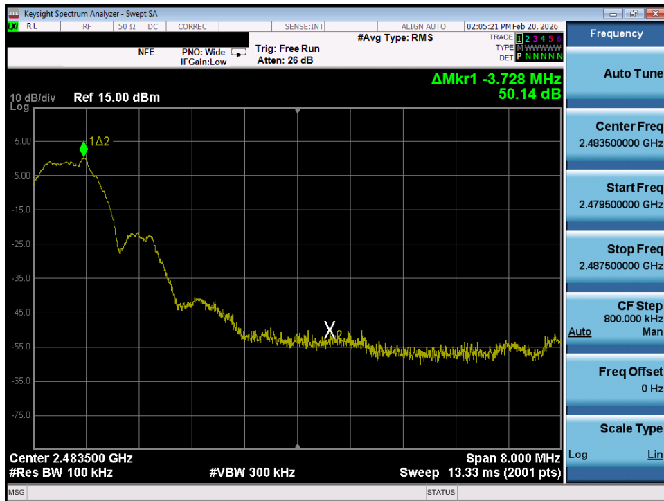
Plot 7-26. Band Edge Plot (ANT+ – Ch. 79)
