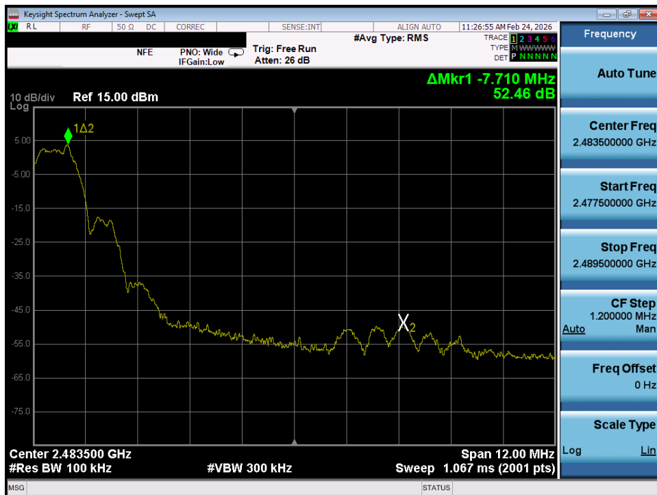
Plot 7-24. Band Edge Plot (ANT+ – Ch. 77)
