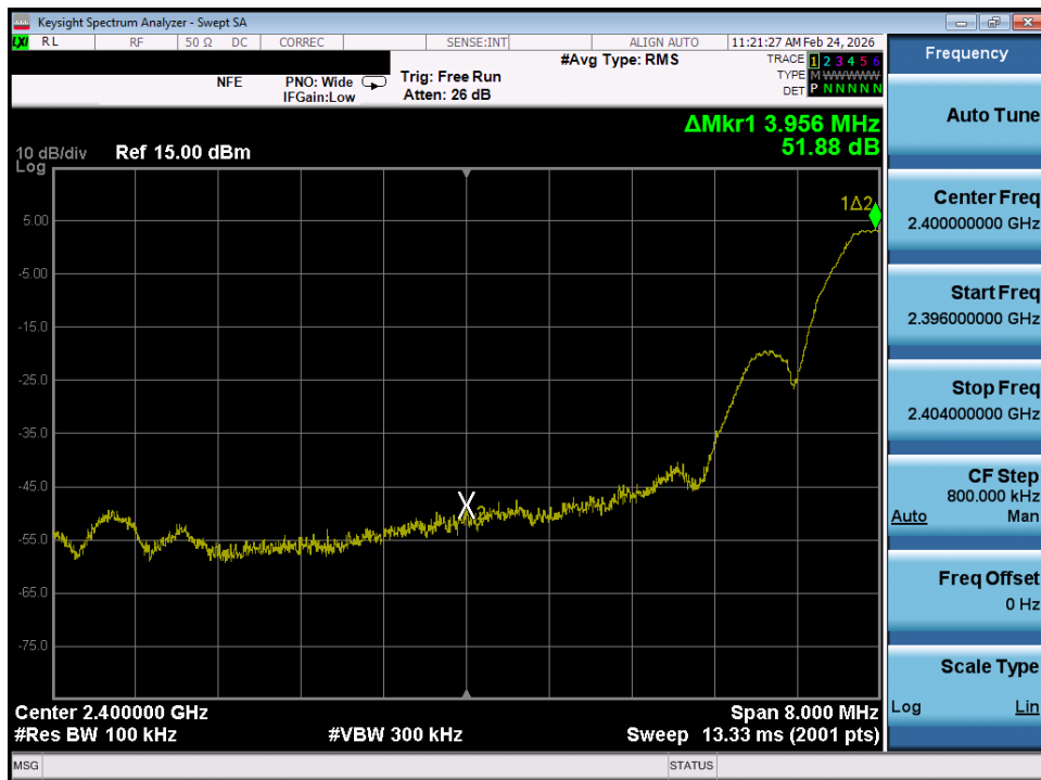
Plot 7-23. Band Edge Plot (ANT+ – Ch. 3)
