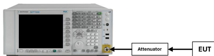
Figure 7-7. Test Instrument & Measurement Setup
