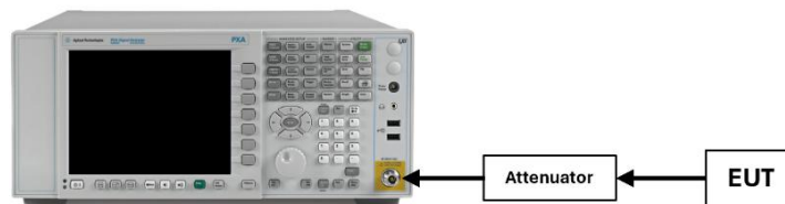
Figure 7-6. Test Instrument & Measurement Setup
