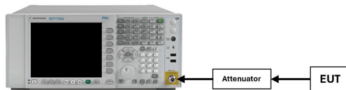
Figure 7-5. Test Instrument & Measurement Setup
