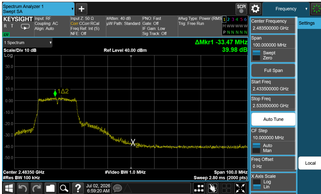
Plot 7-23. Band Edge Plot (802.11g – Ch. 9)
