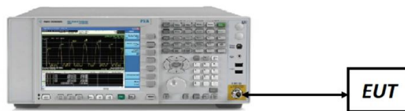
Figure 7-3. Test Instrument & Measurement Setup
