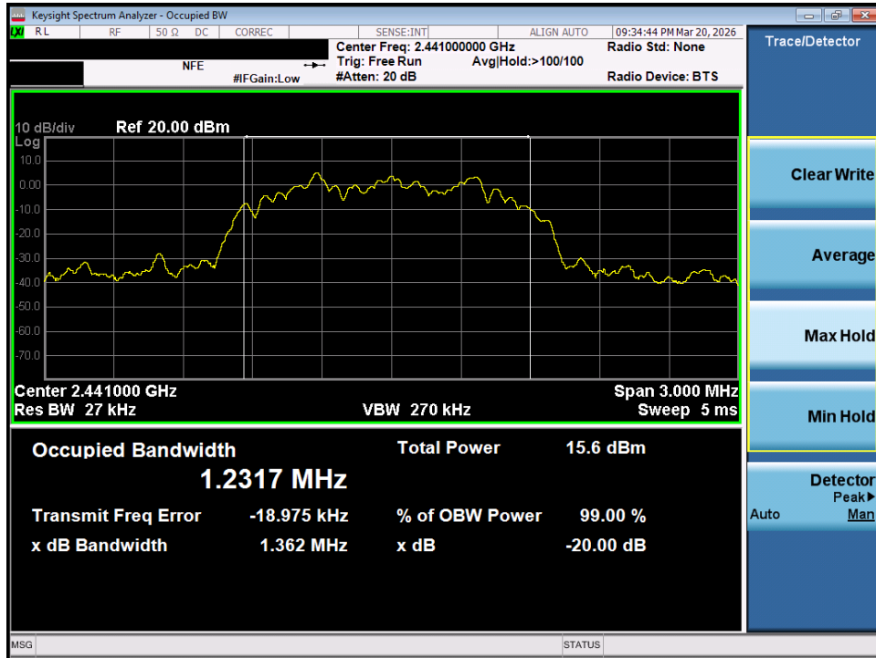
Plot 7-8. 20dB Bandwidth Plot (Bluetooth, 3Mbps – Ch. 39)
