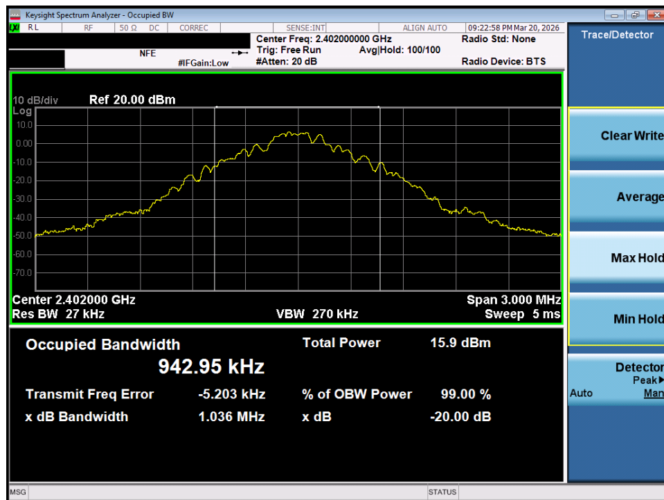
Plot 7-1. 20dB Bandwidth Plot (Bluetooth, 1Mbps – Ch. 0)
