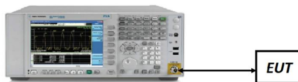
Figure 7-1. Test Instrument & Measurement Setup
