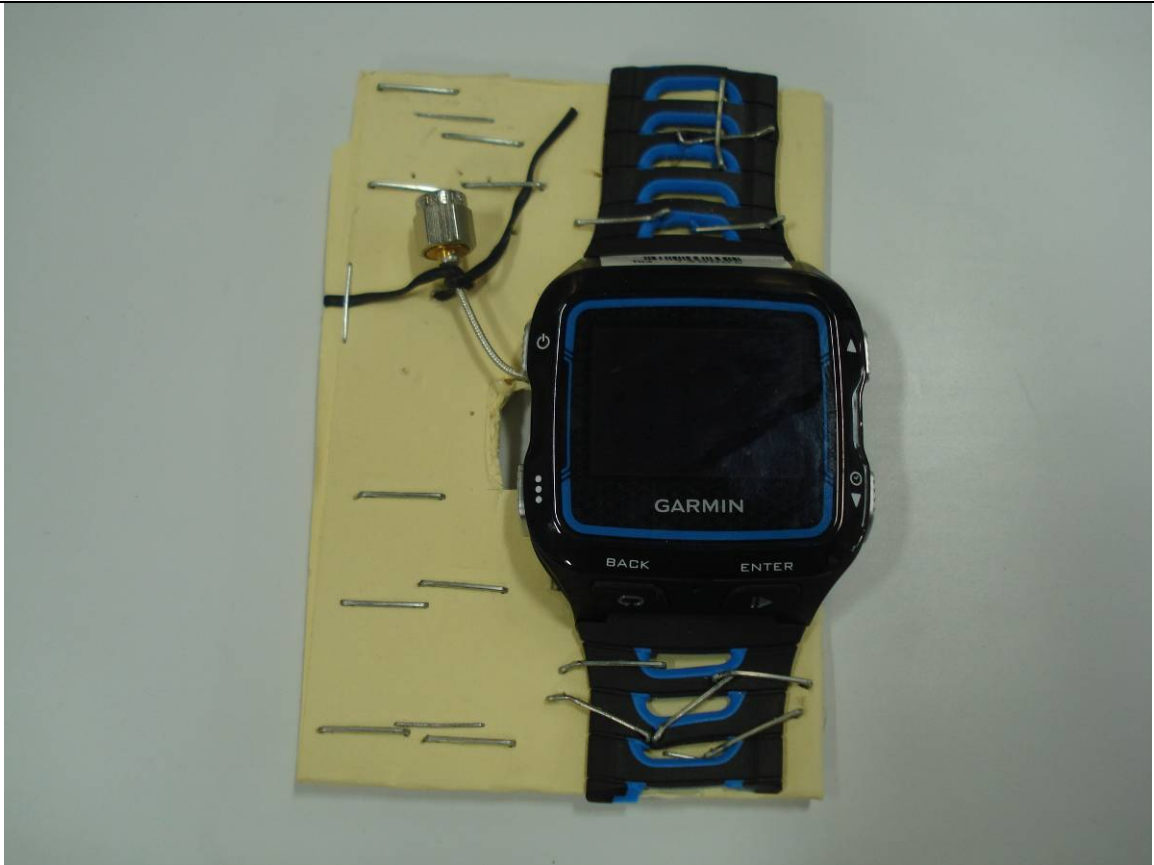
Unit Modified for Conducted Power
