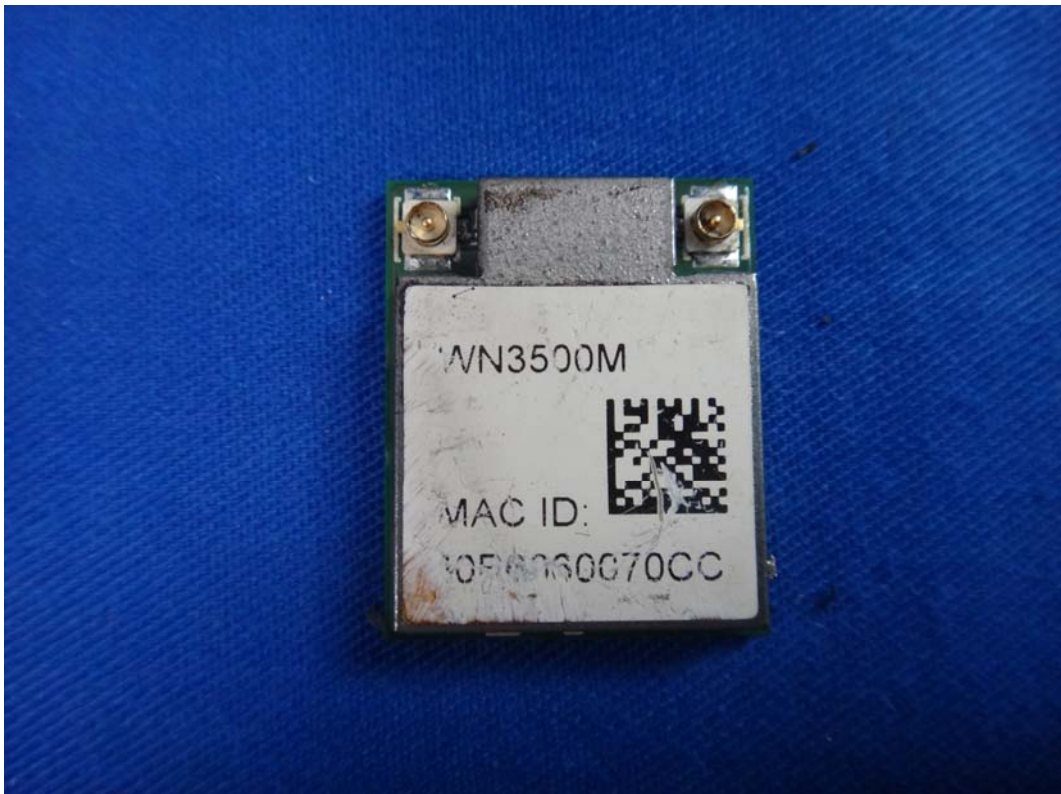
(19) EUT Photo-WLAN Modulw
