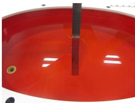
Liquid depth in the flat Phantom ( \geq 15\text{cm} depth) HSL(2450MHz) HSL(5GHz)
