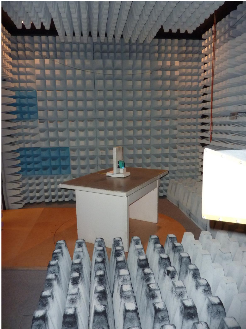
136258_d.JPG: IUH-F190-V1-FR2-02, test set-up fully anechoic chamber
