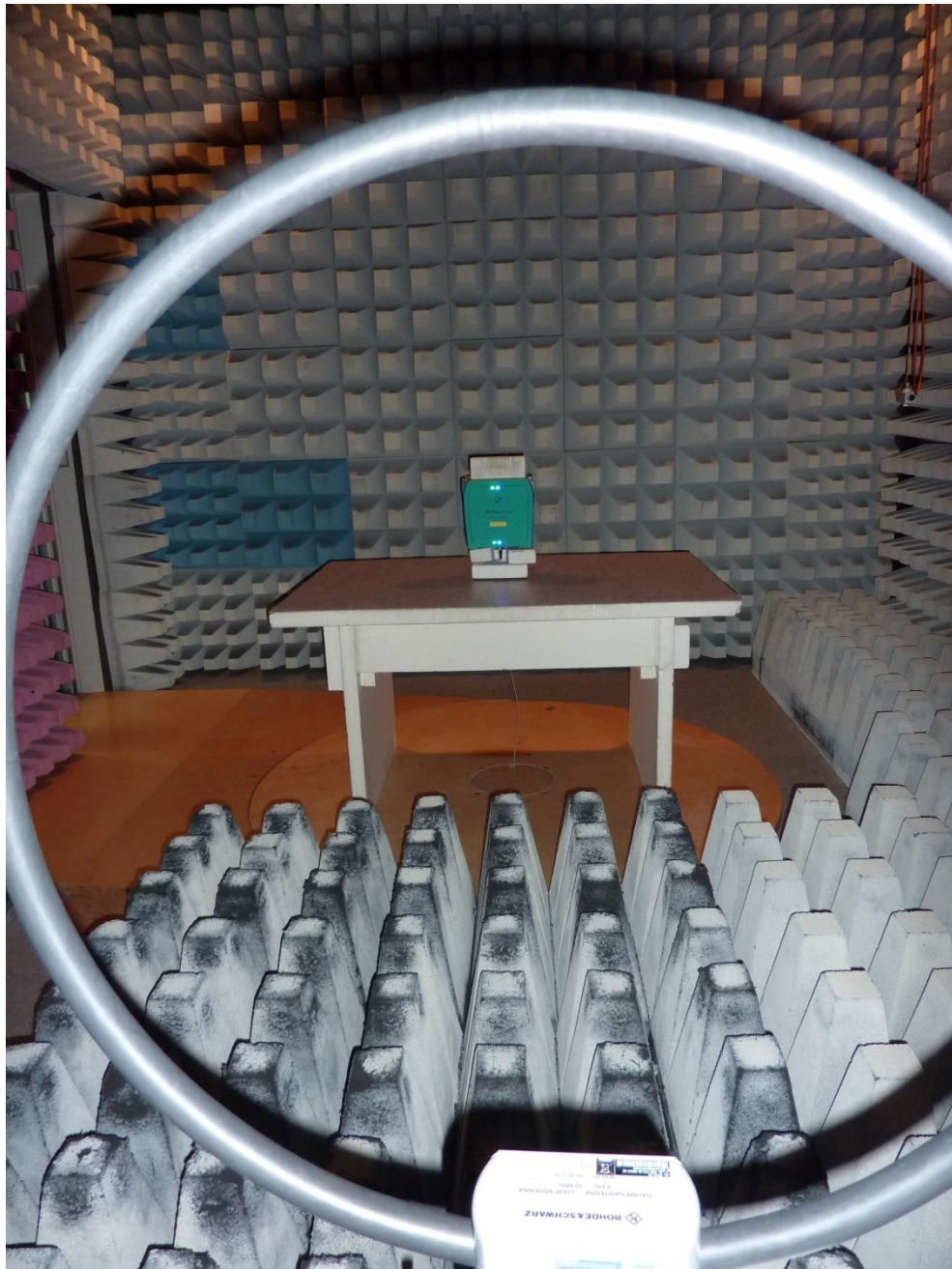
152117_e.JPG: IUH-F192-V1-FR2-02, test setup fully anechoic chamber
