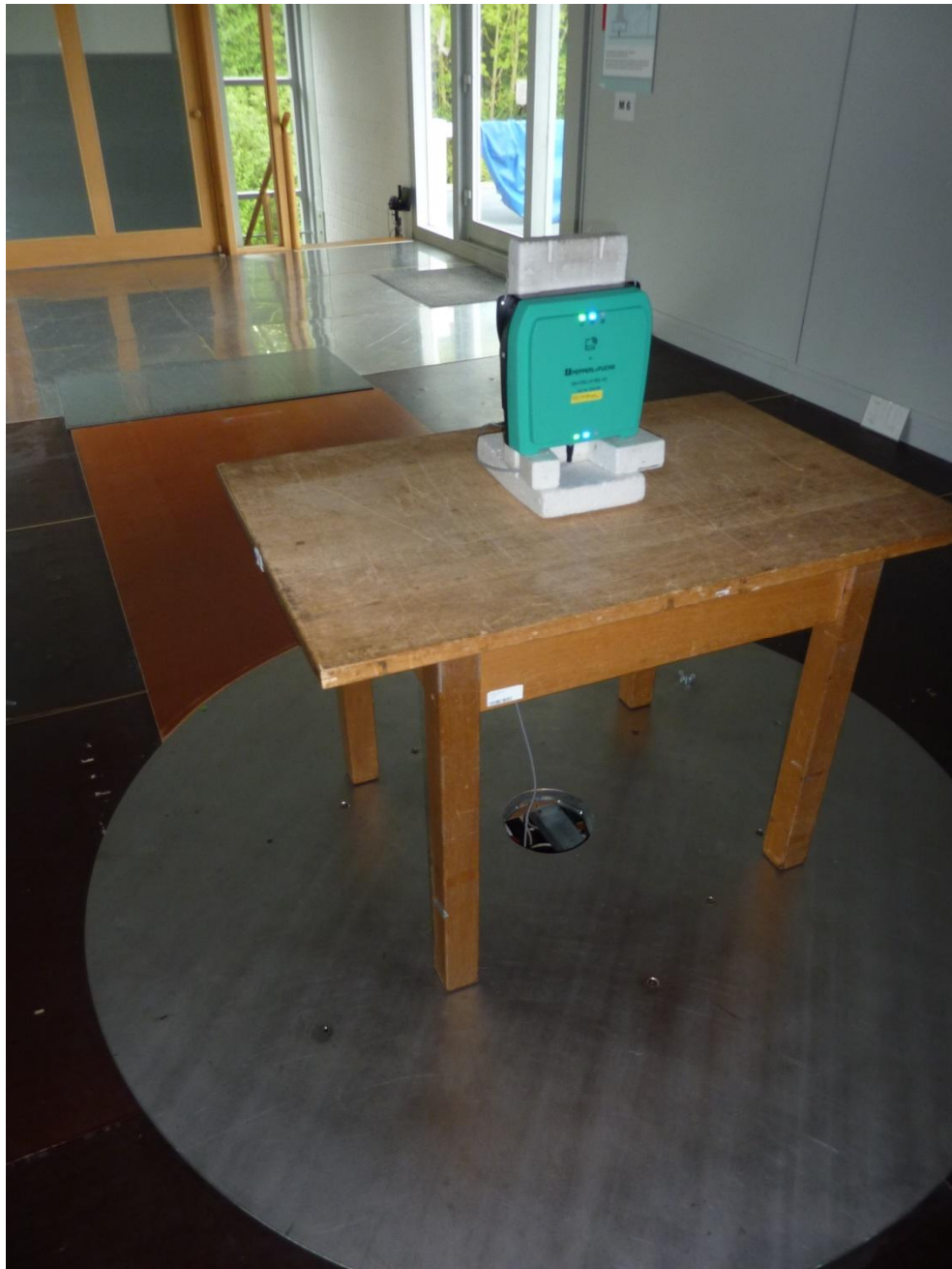
152117_g.JPG: IUH-F192-V1-FR2-02, test set-up open area test site
