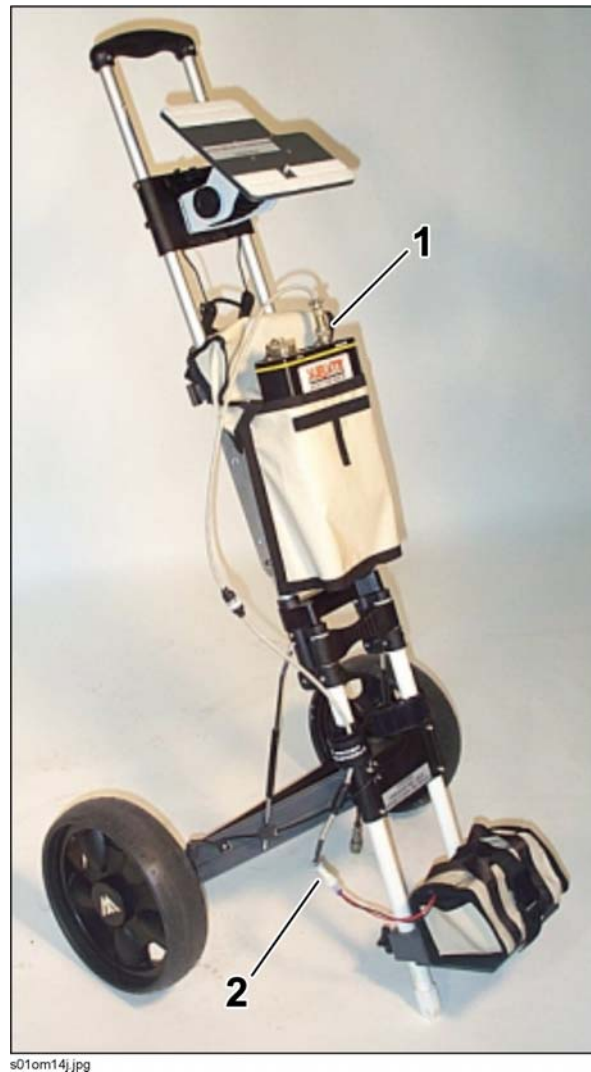
Fig. 4-4 – Battery and cabling support
