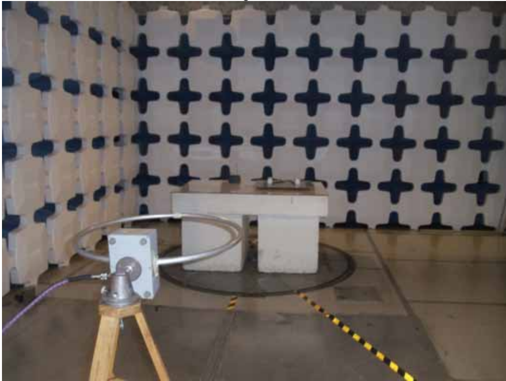
Test Setup for Radiated Emissions, Below 1GHz – Horizontal Polarization With M190-A3 external antenna
