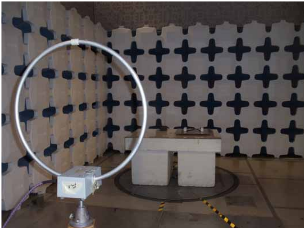
Test Setup for Radiated Emissions, Below 1GHz – Vertical Polarization With M190-A3 external antenna
