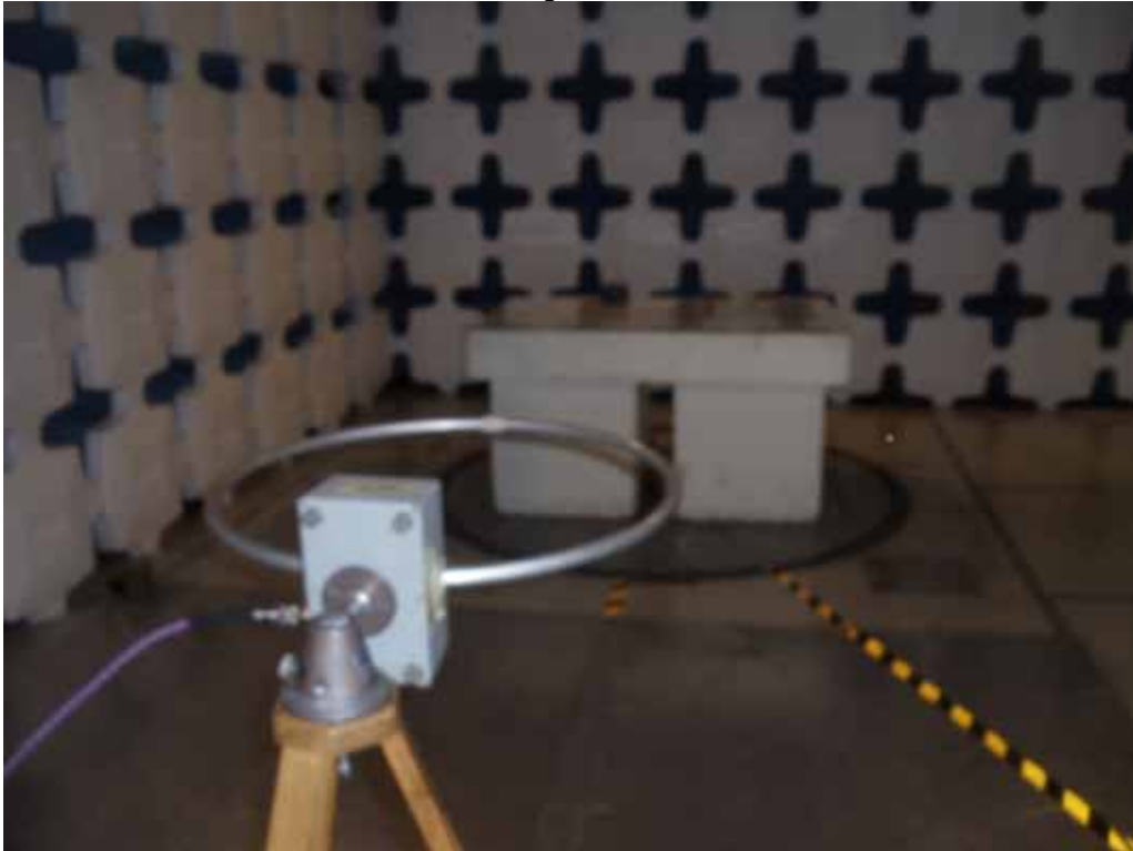
Test Setup for Radiated Emissions, Below 1GHz – Horizontal Polarization With M190-A2 external antenna
