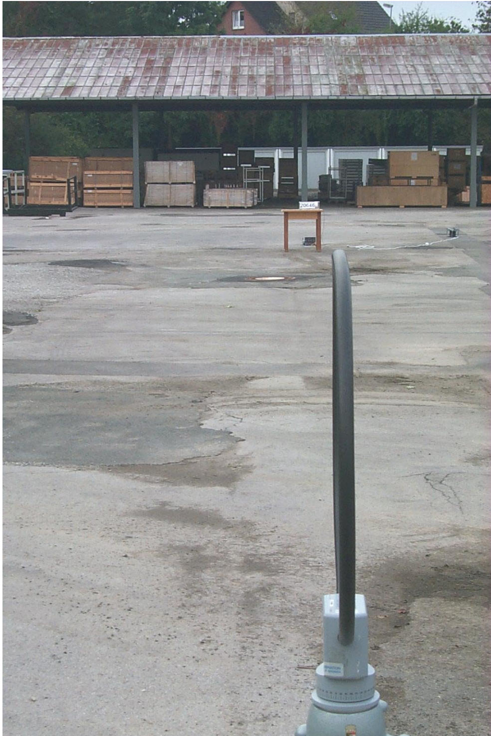
20646_g.jpg test set-up final emission measurement (9 kHz to 30 MHz)
