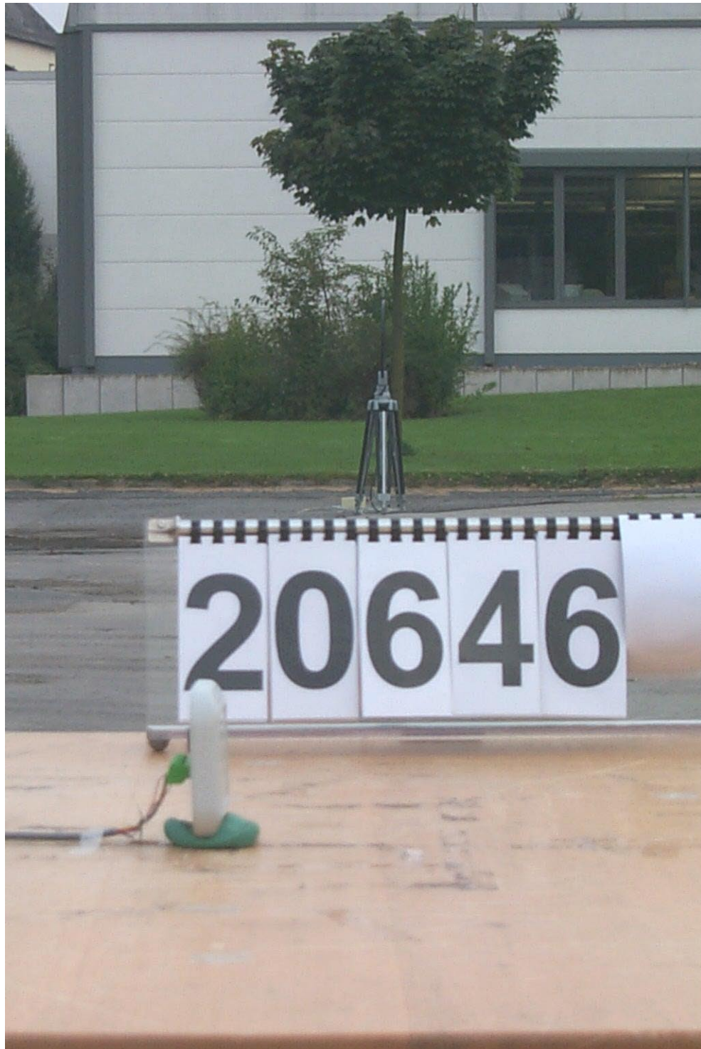
20646_f.jpg test set-up final emission measurement (9 kHz to 30 MHz)
