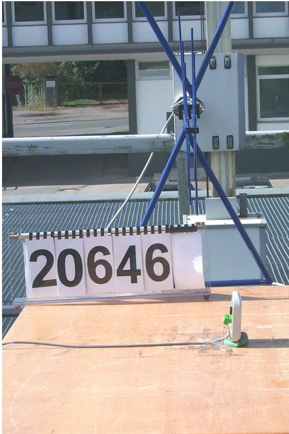
20646_e.jpg test set-up final emission measurement (30 MHz to 1 GHz)
