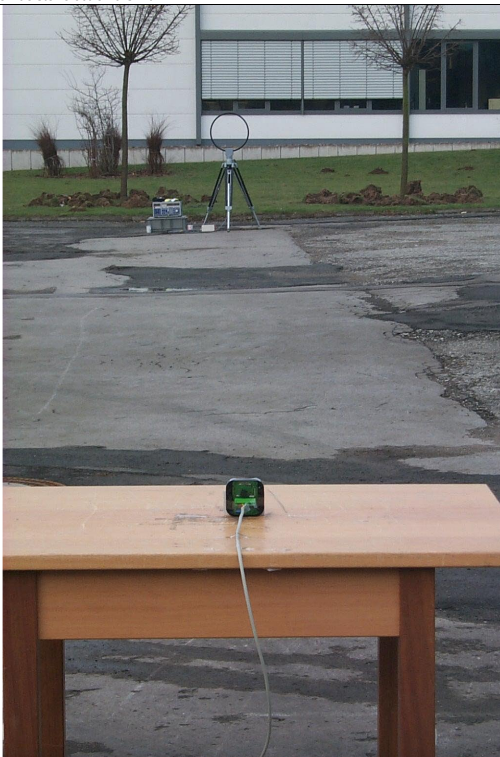
30013_11.jpg Test set-up final emission measurement (9 kHz to 30 MHz)
