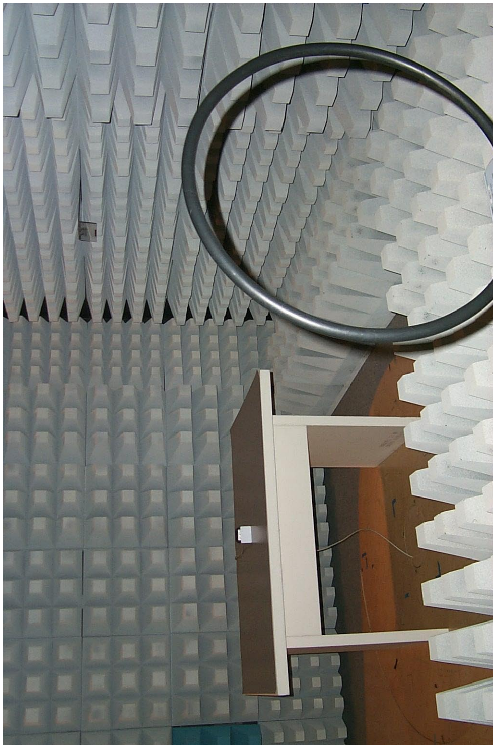
30013_6.jpg Test set-up preliminary emission measurement (9 kHz to 30 MHz)
