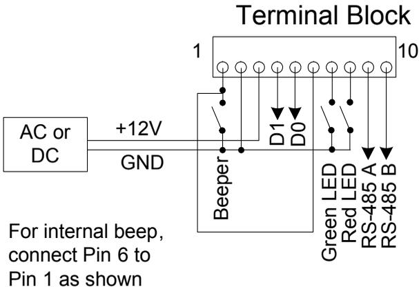
FIGURE 2. Beeper Wiring
