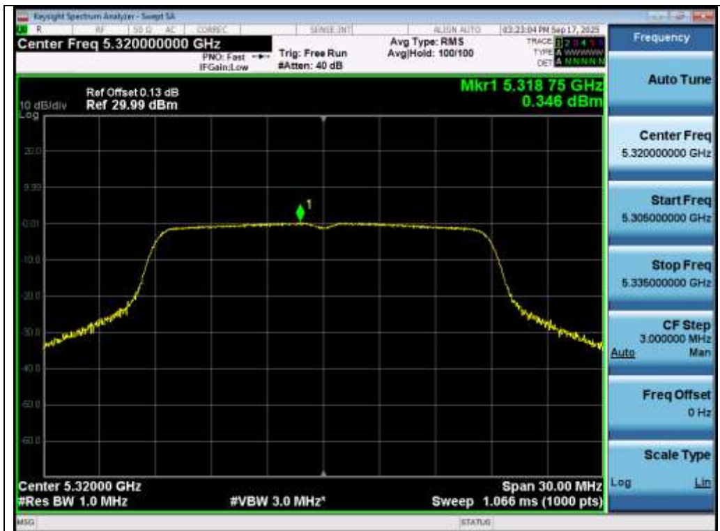
Test_Graph_802.11ac20_ANT1_5320_MCS0_PSD
