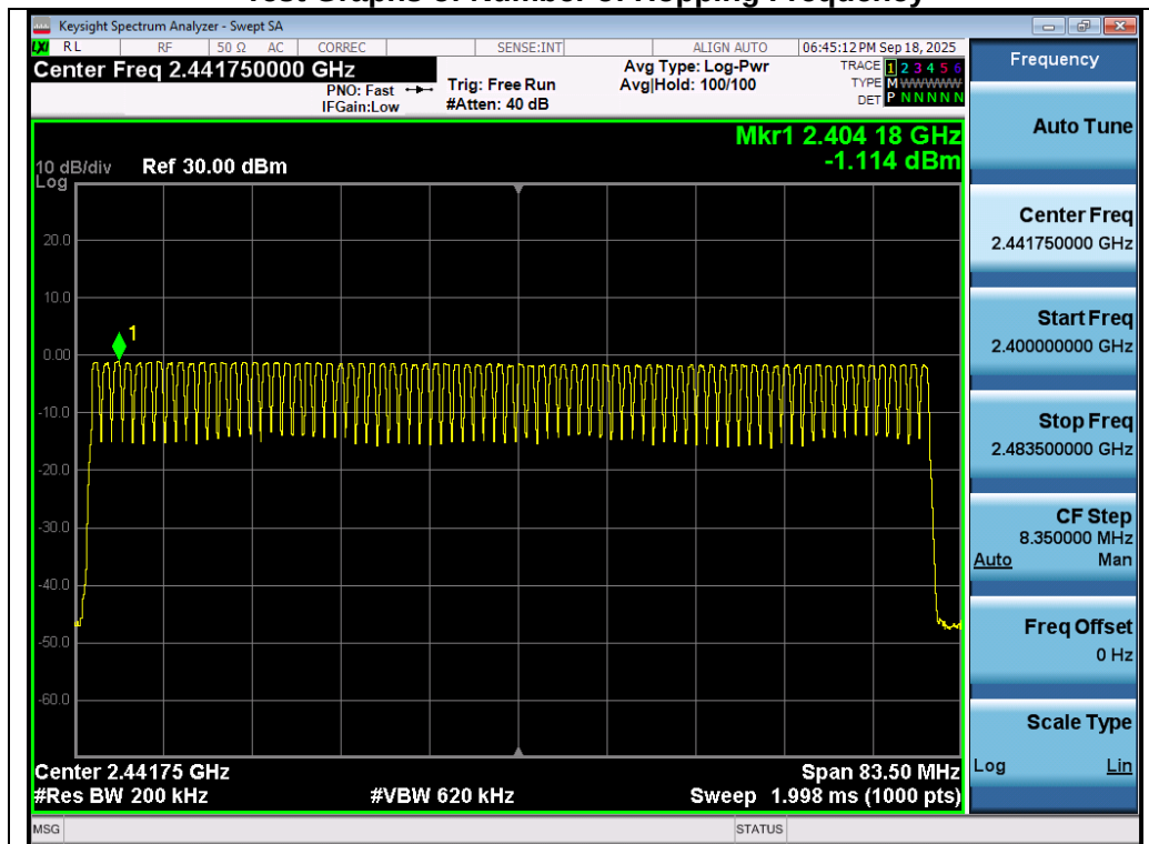
Test_Graph_BR_HOP_ANT1_NA_1Mbps_Number of Hopping
