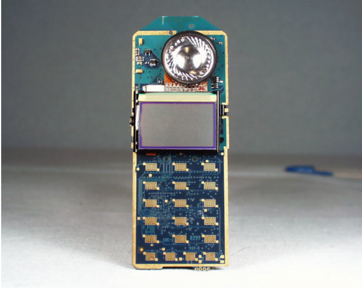
Inside View - Side A with LCD display installed
