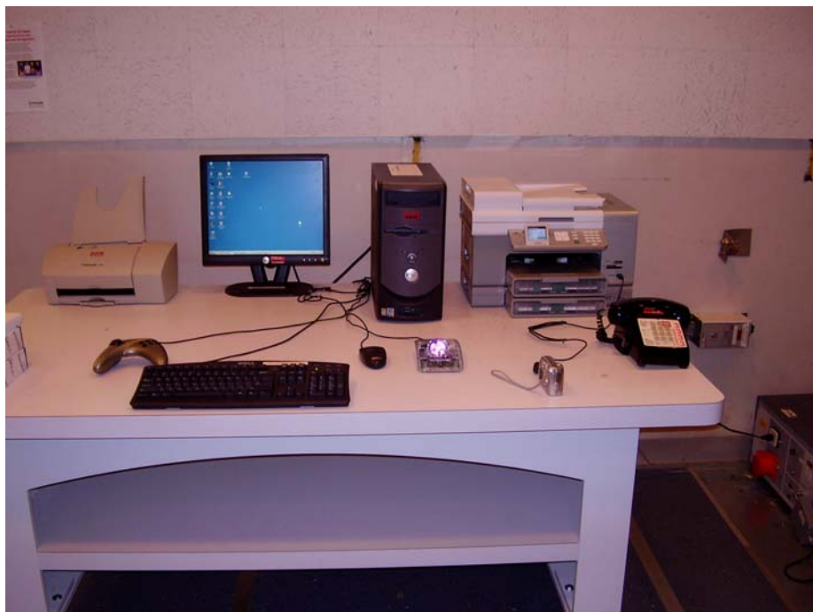
Figure 7. Test configuration for transmitter conducted emissions (front view).
