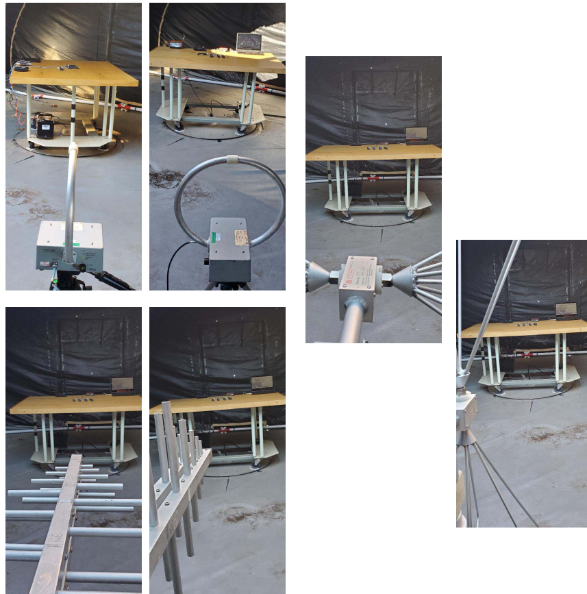
Figure 4: Radiated Emissions Test Setup Photograph(s).
