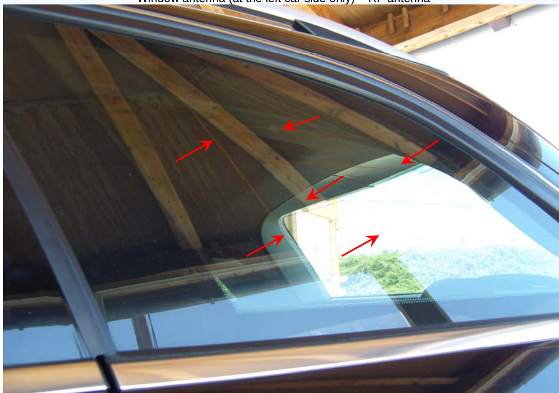
Window antenna (at the left car side only) – RF antenna
