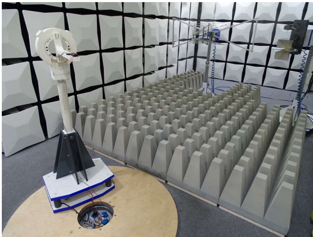
Photo 3: Test setup for radiated measurements above 1 GHz
