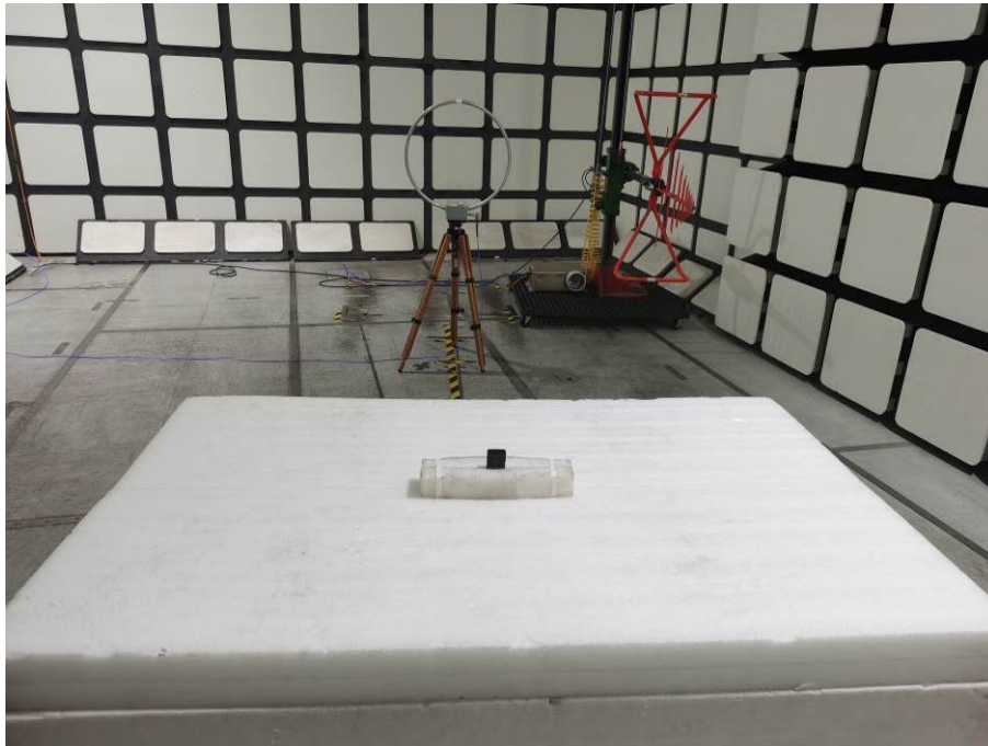
Radiated EmissionsView (Below 30MHz)
