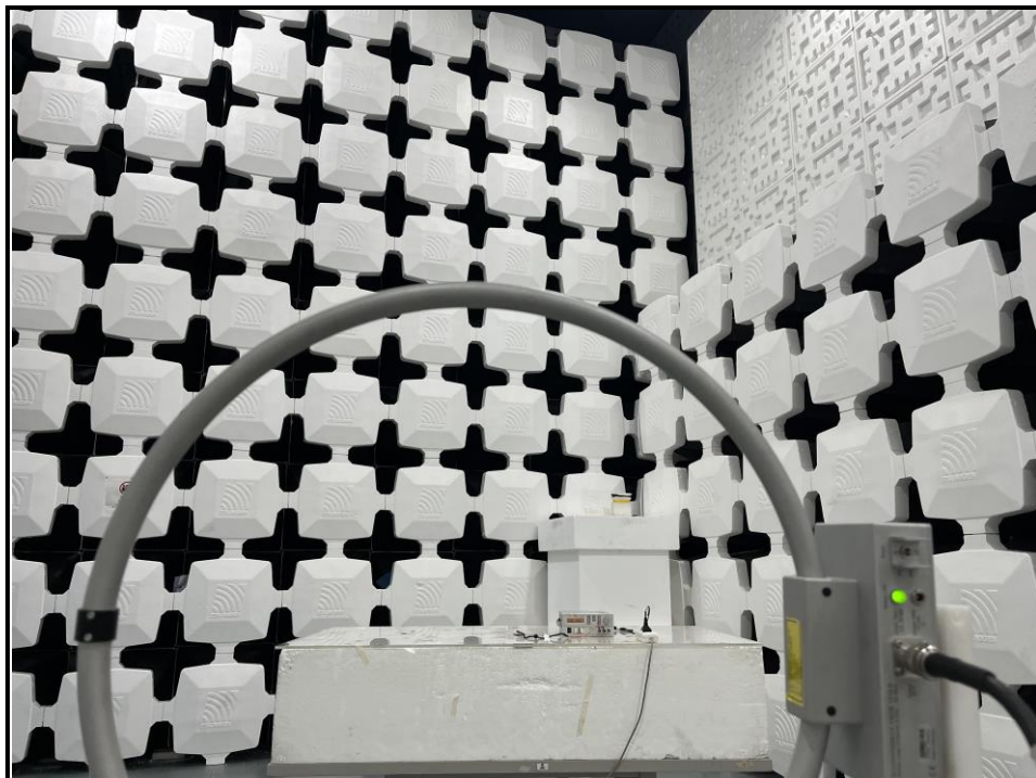
Fig. 1 Radiated emission setup photo(Below 30MHz)
