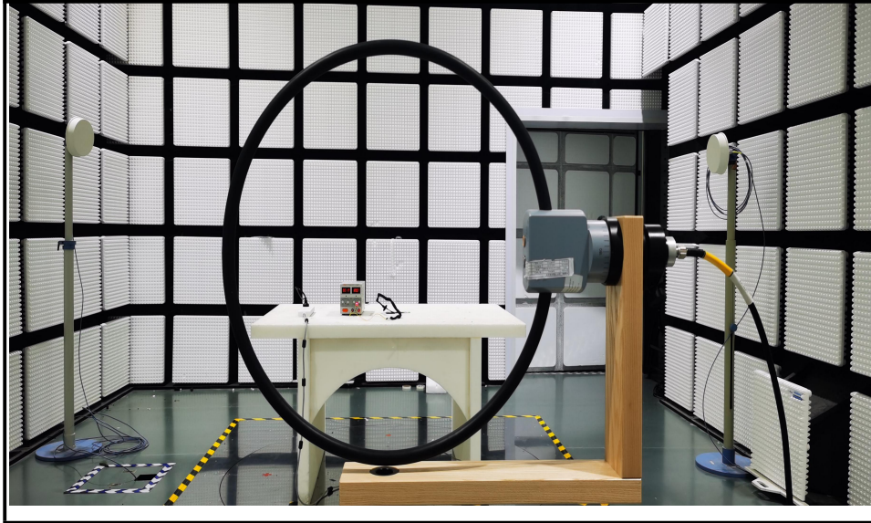
Fig. 1 Radiated emission setup photo(Below 30MHz)
