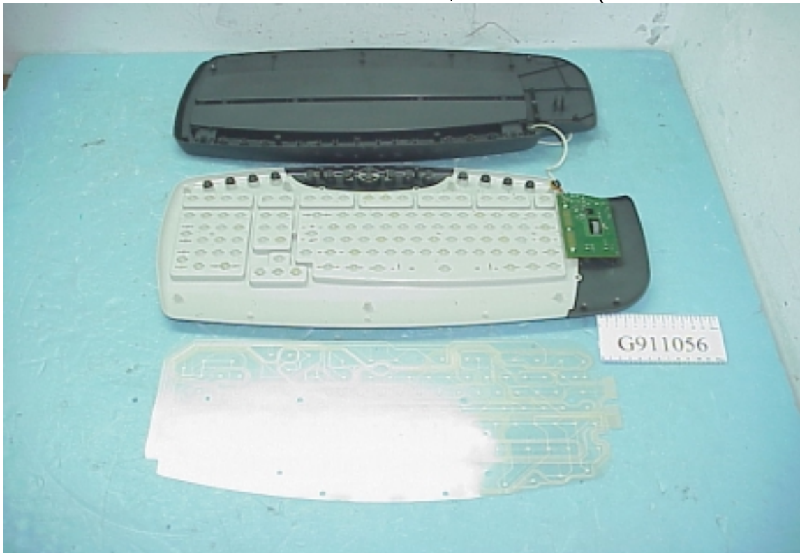
Figure 4 M/N OFFICE 800, Internal View (Removed LED / Control Board)
