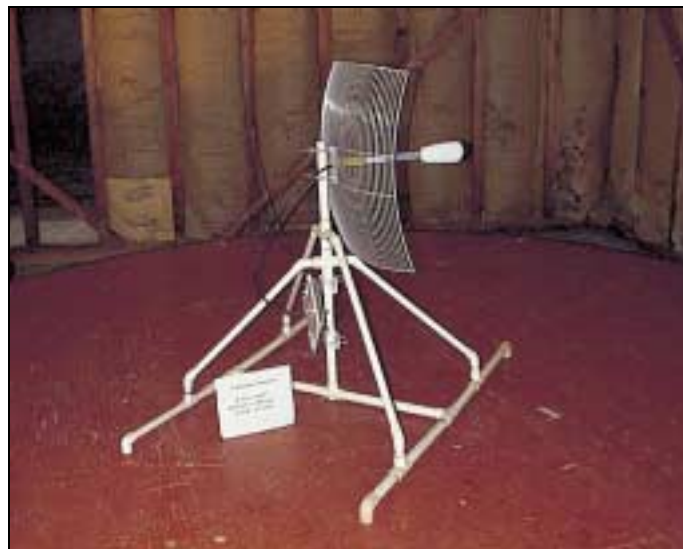
Transmitter with Parabolic Antenna
