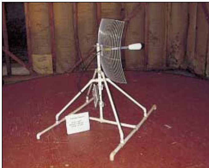
Transmitter with Parabolic Antenna
