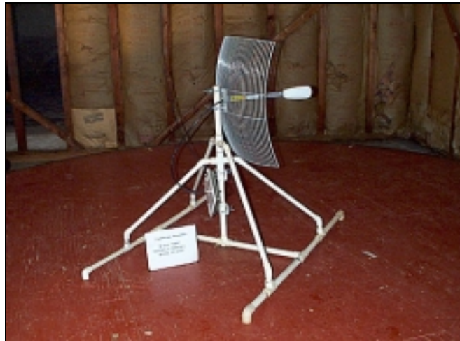
Transmitter with Parabolic Antenna
