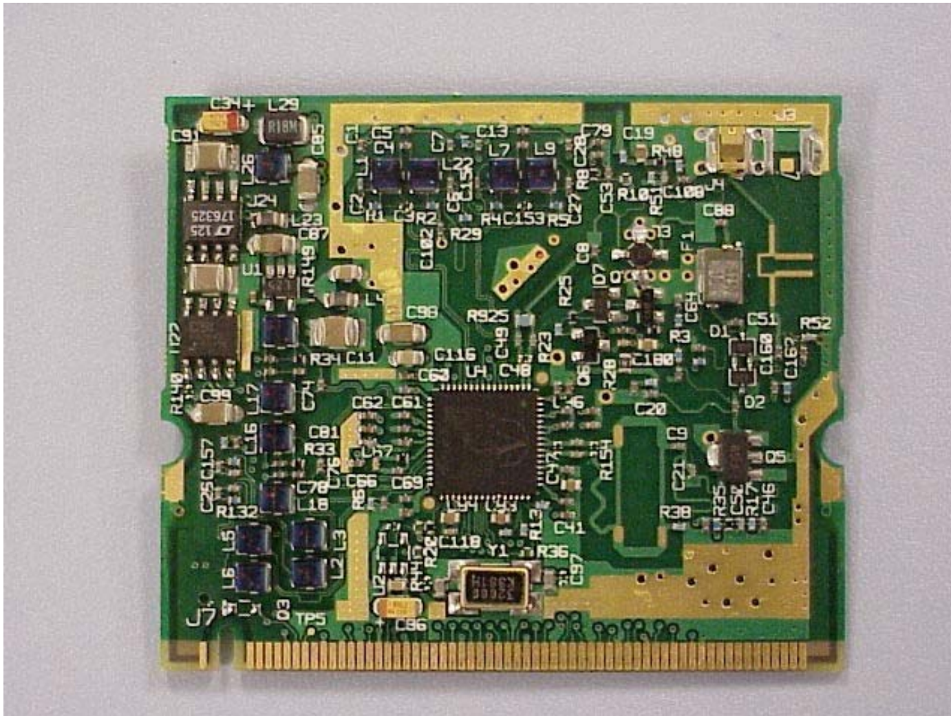
Front Side of 5 GHz MINI PCI W/ Atheros Chip Set Shield removed
