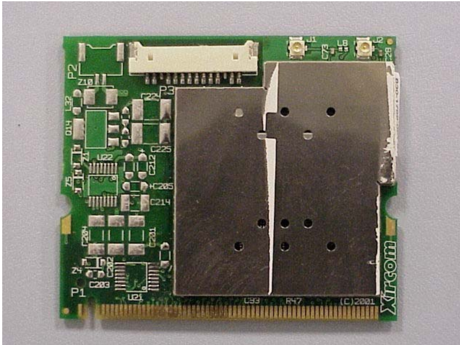
2.4 GHz MINI PCI card front side with shield
