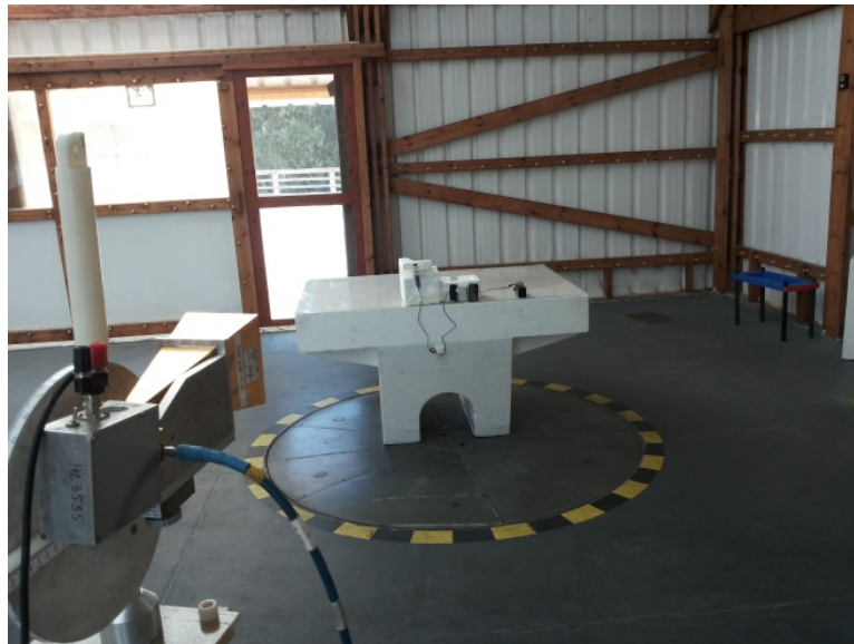
Photograph 8.1.4 Setup for final radiated emission measurements, EUT cabling
