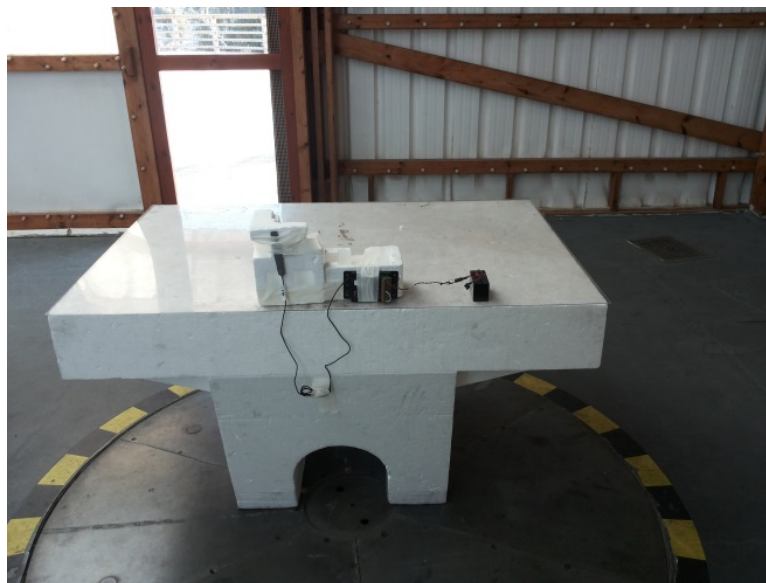
Photograph 8.1.4 Setup for final radiated emission measurements, EUT cabling
