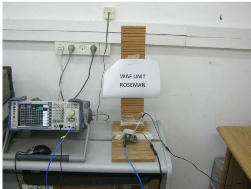
Figure 3. Conducted Emission From Antenna Ports Test
