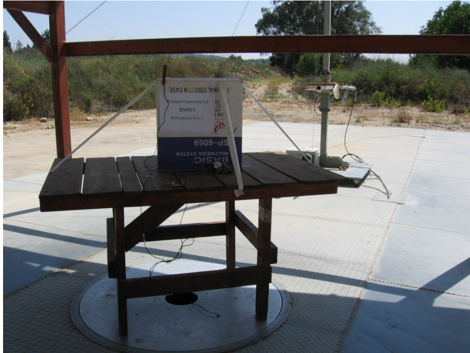
Figure 2. Radiated Emission Test Aviv 3 Antenna
