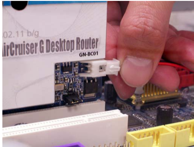
Figure 2-4 – Attach AirCruiser G power connector
