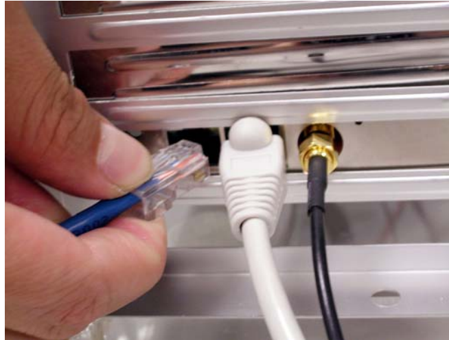
Figure 3-2 – LAN (network) cable for initial setup. The other end will go into your Notebook PC or Desktop NIC.
