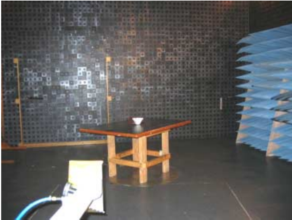
Photograph No.3 Radiated emission measurement test setup from 1 to 18 GHz
