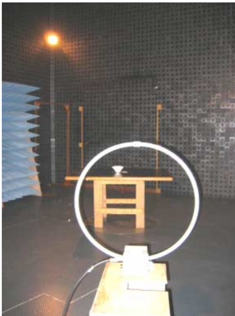
Photograph No.1 Radiated emissions measurement test setup below 30 MHz
