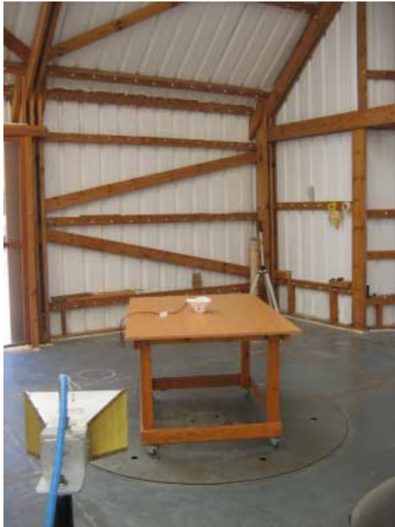
Photograph No.6 Band edge emission measurement setup
