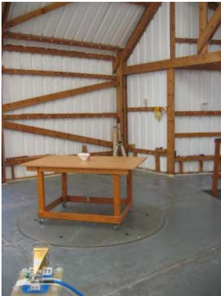
Photograph No.4 Radiated emission measurement test setup from 26.5 to 40 GHz
