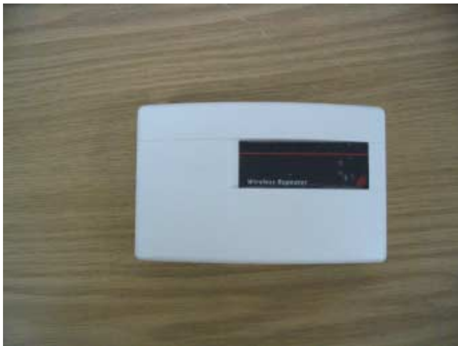
Photograph No.1 RP296EWR0USA repeater front view
