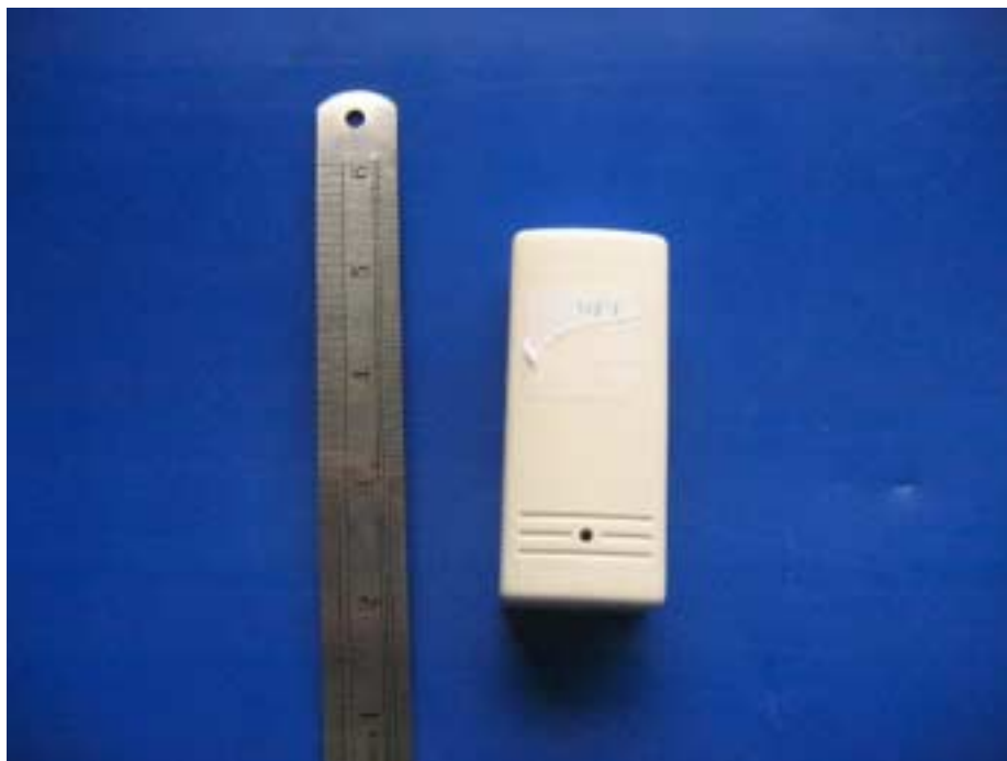
Photograph No.1 RWT71M433USA transmitter front view
