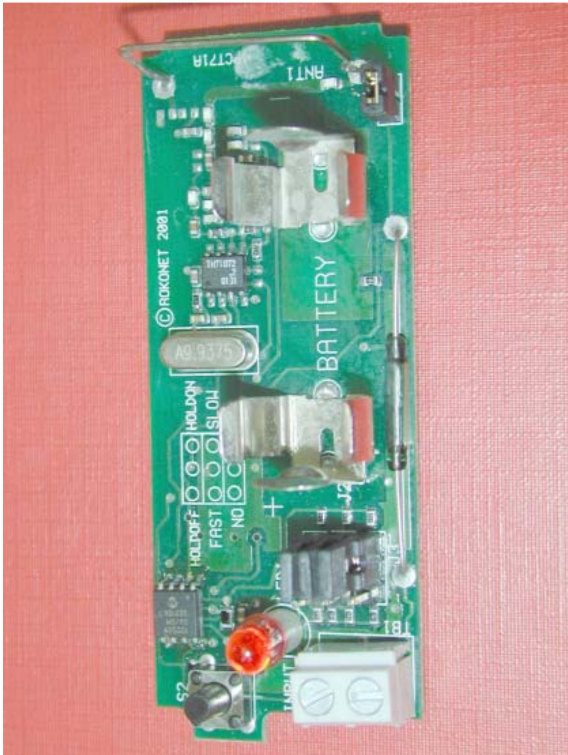
Photograph No.3 RWT71V2 detector PCB front view
