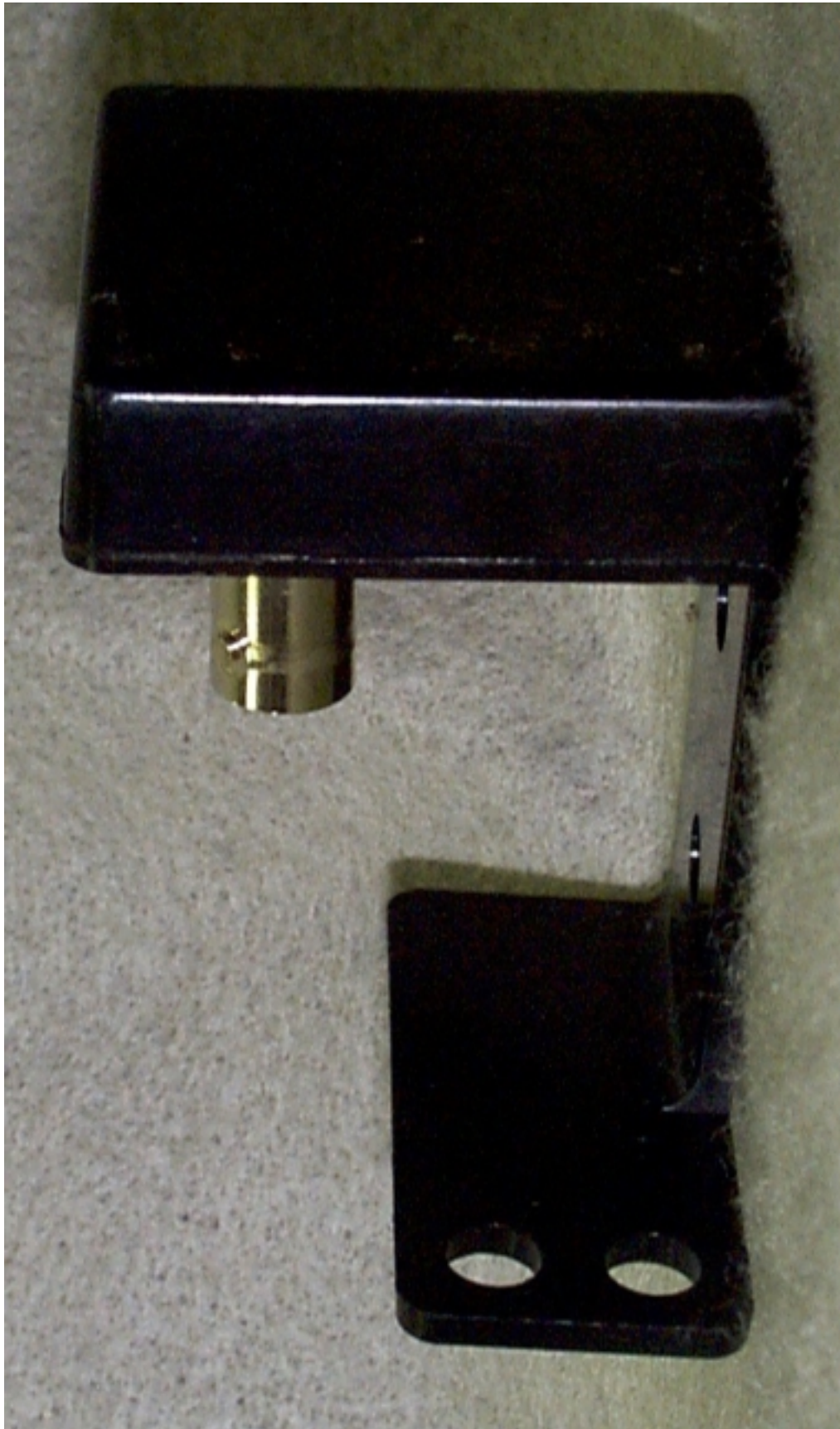
Photo 13. Top View of Receive Antenna – Type 1 (Patch w/ LNA)
