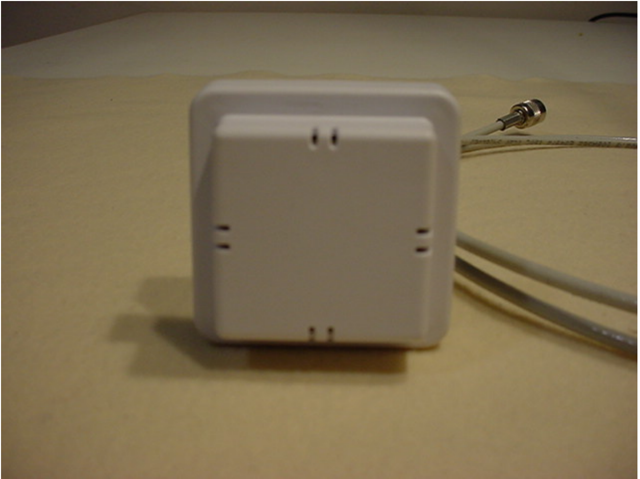
Figure 8: Transmit Antenna Front
