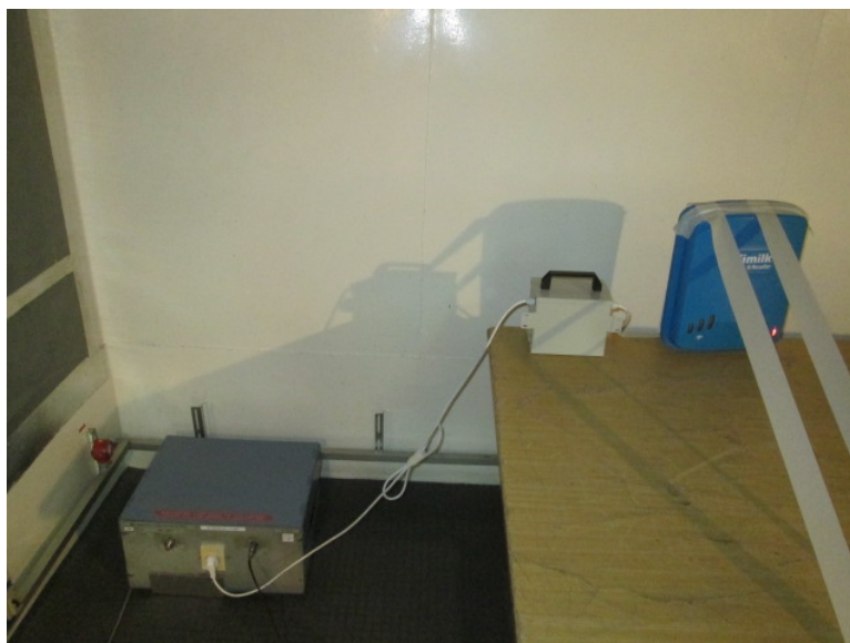
Photograph 8.1.1 Setup for conducted emission measurements
