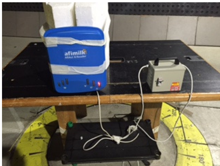
Photograph 8.2.2 Setup for radiated emission measurements, EUT cabling
