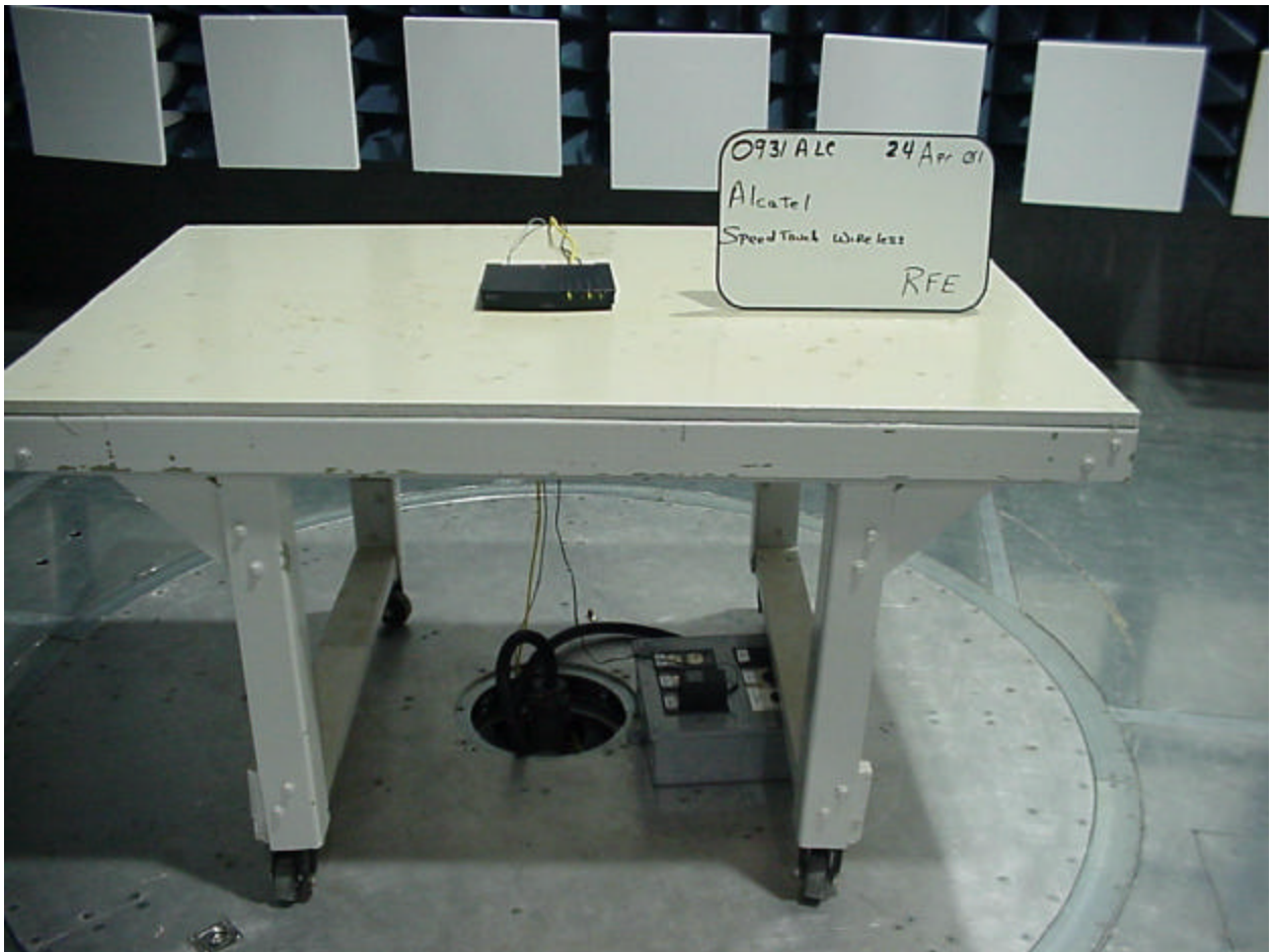
Figure 1 - Preliminary Radiated Emissions Test Setup (Chamber - Front)
