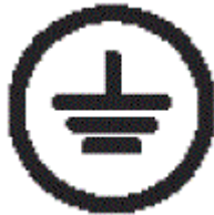
Figure 8 Equipment connection to earth
