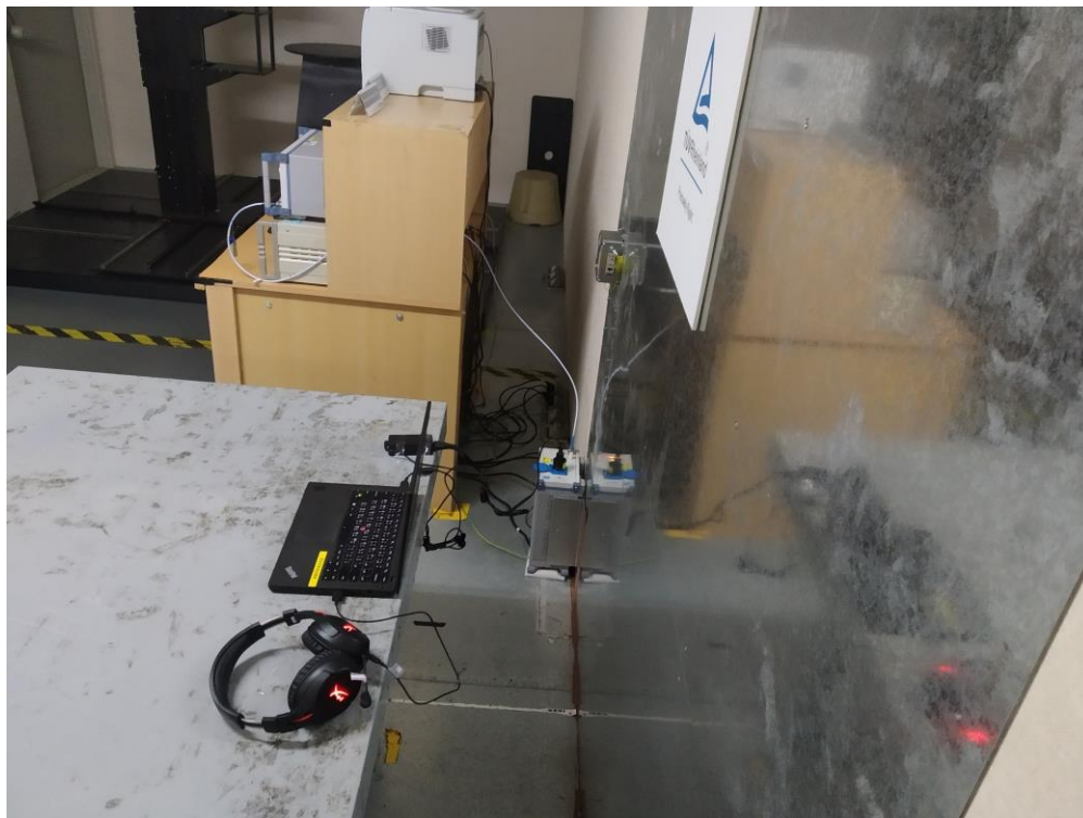
Photograph 8: Set-up for Mains Conducted Testing (Back View)
