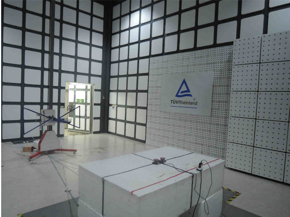
Photograph 3: Set-up for Spurious Emissions (Back View 2)
