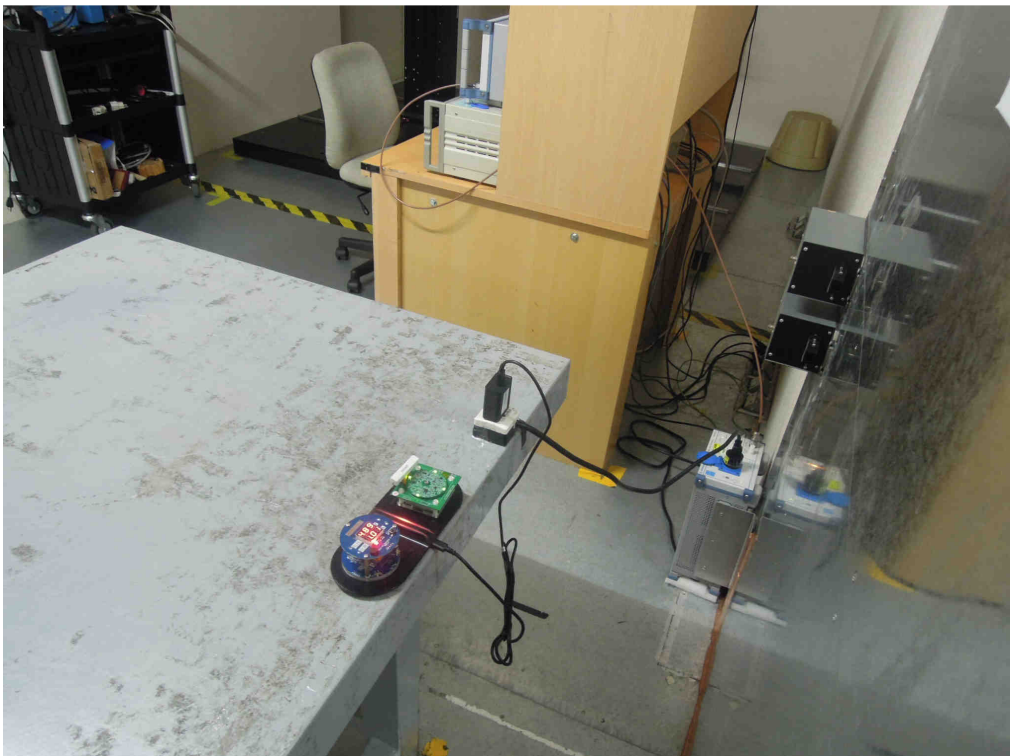
Photograph 4: Set-up for for Mains Conducted testing Back
