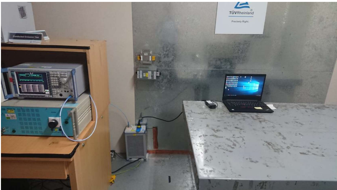
Photograph 5: Set-up for for Mains Conducted testing Front
