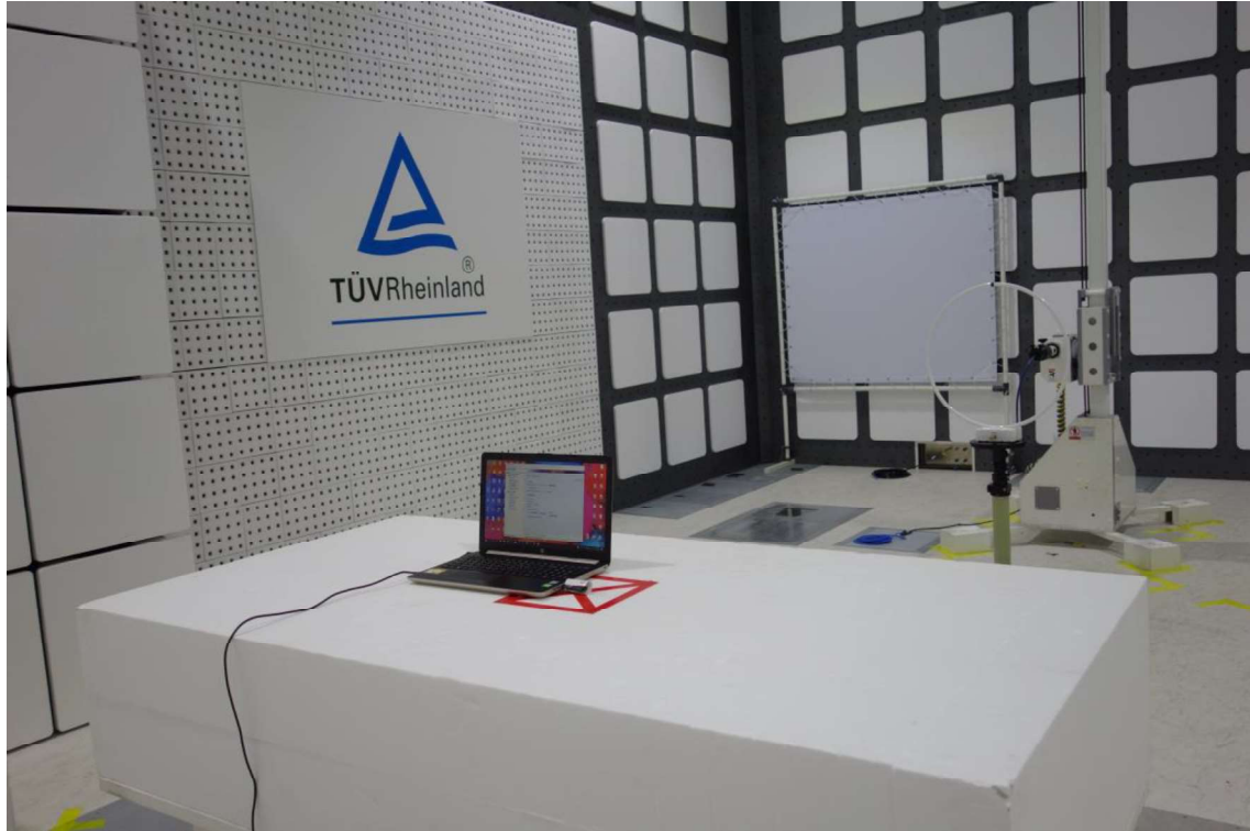
Photograph 2: Set-up for Spurious Emissions (Back View 1)
