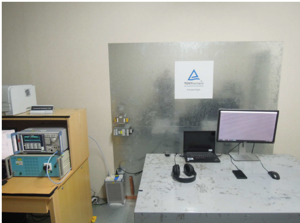
Photograph 9: Set-up for for Mains Conducted testing Front
