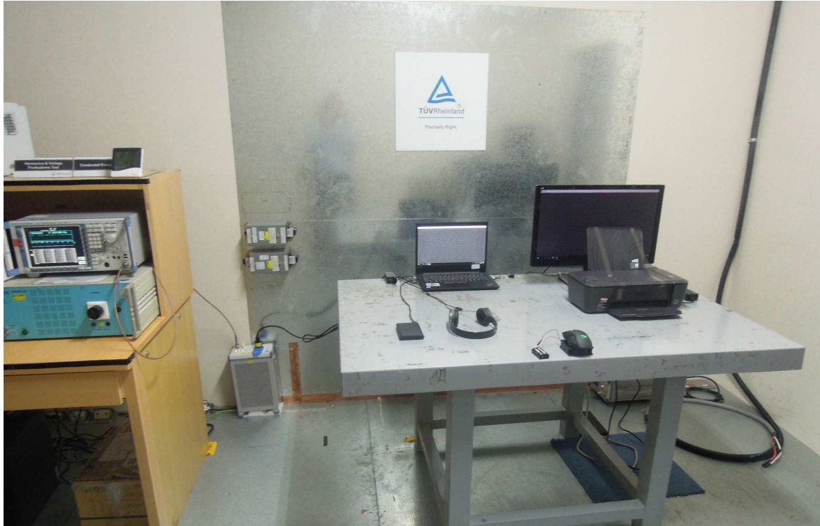
Photograph 6: Set-up for for Mains Conducted testing Front
