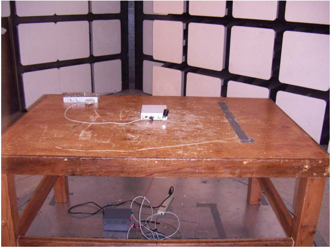
Radiated test set-up
